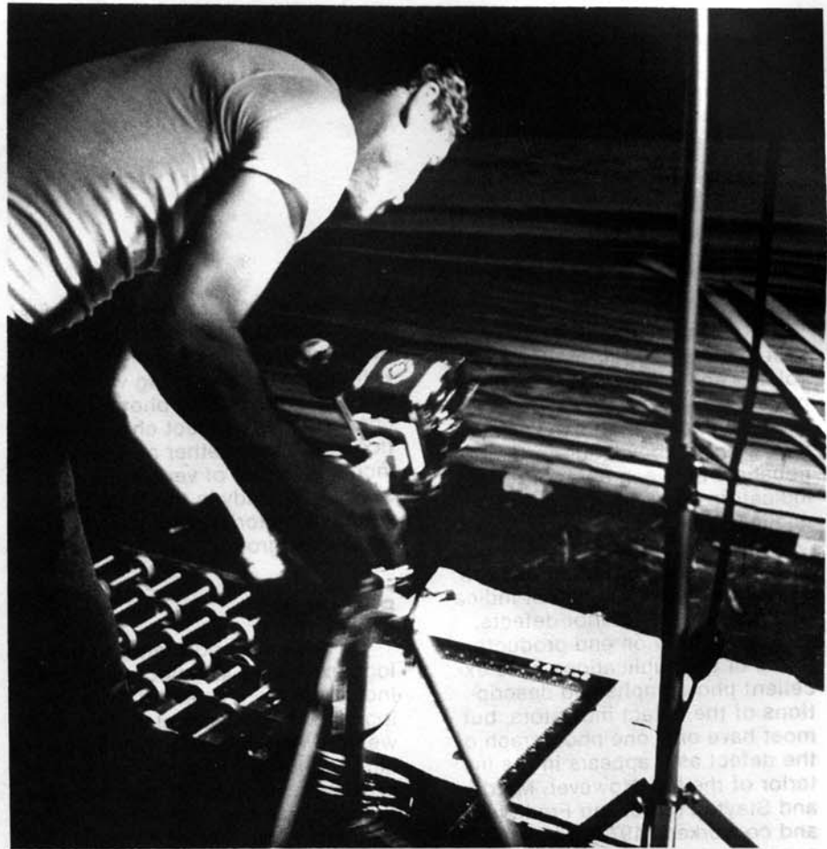
Figure 2.—Photography setup showing camera, dead rolls for moving veneer, and square used to outline and show defect size. Magnetic numbers were placed on square to correlate log and defect to each photograph.
