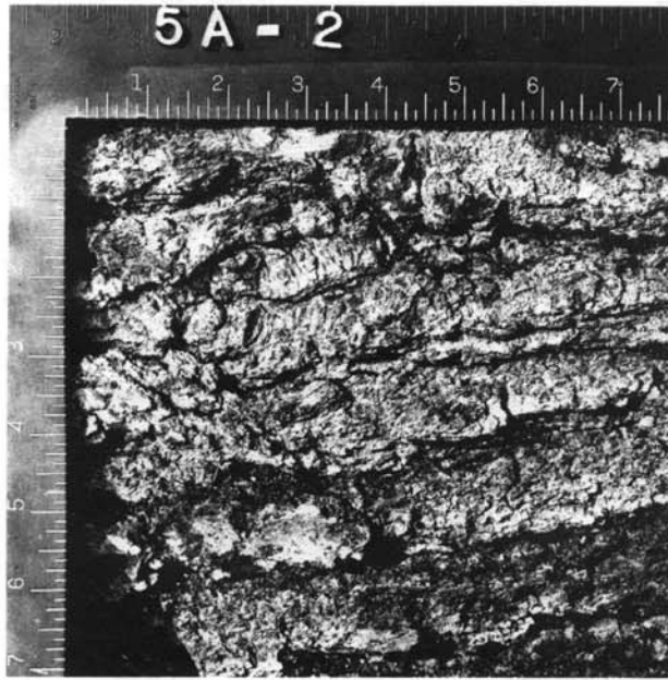
Defect size . . . . . 2 1/2 x 2 inches Log diameter at defect . . . . . 22.5 inches Flitch thickness at defect . . . . . 10.1 inches Log position . . . . . upper log
