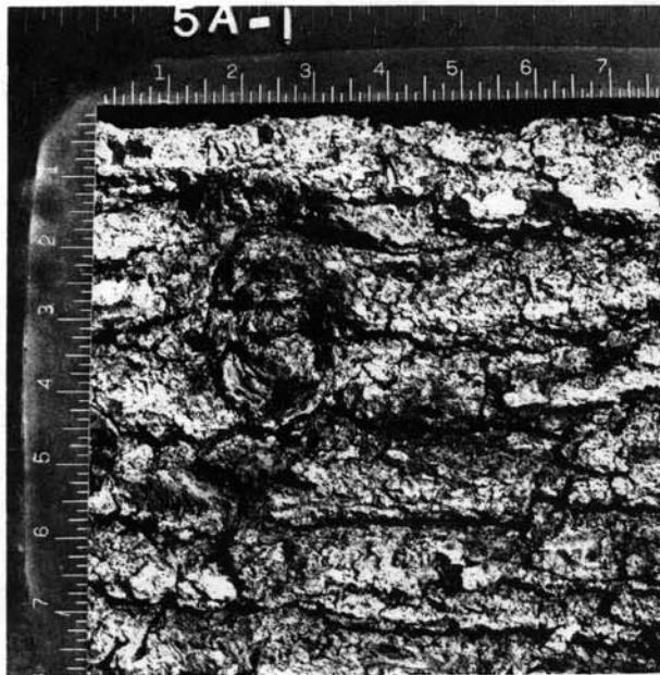
Figure 6.—Knot overgrowth (medium distortion) and associated internal defects.
