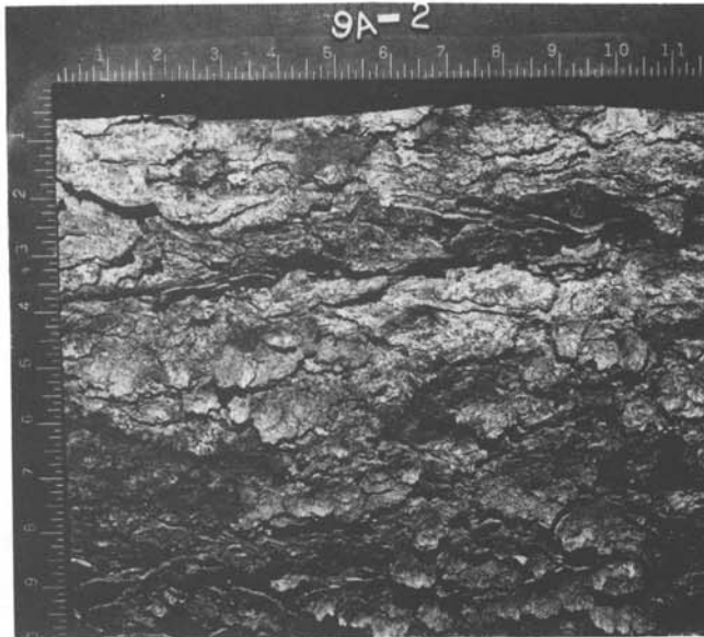
Figure 10.—Overgrown seam and associated internal defects.
