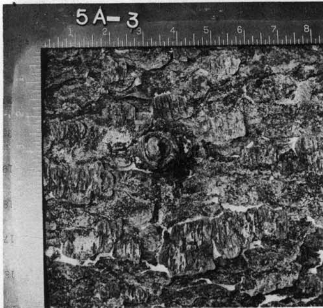
Figure 4.—Suppressed bud cluster and associated internal defects.
