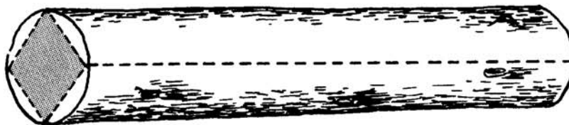
Figure 6.—Selecting the grading face.
