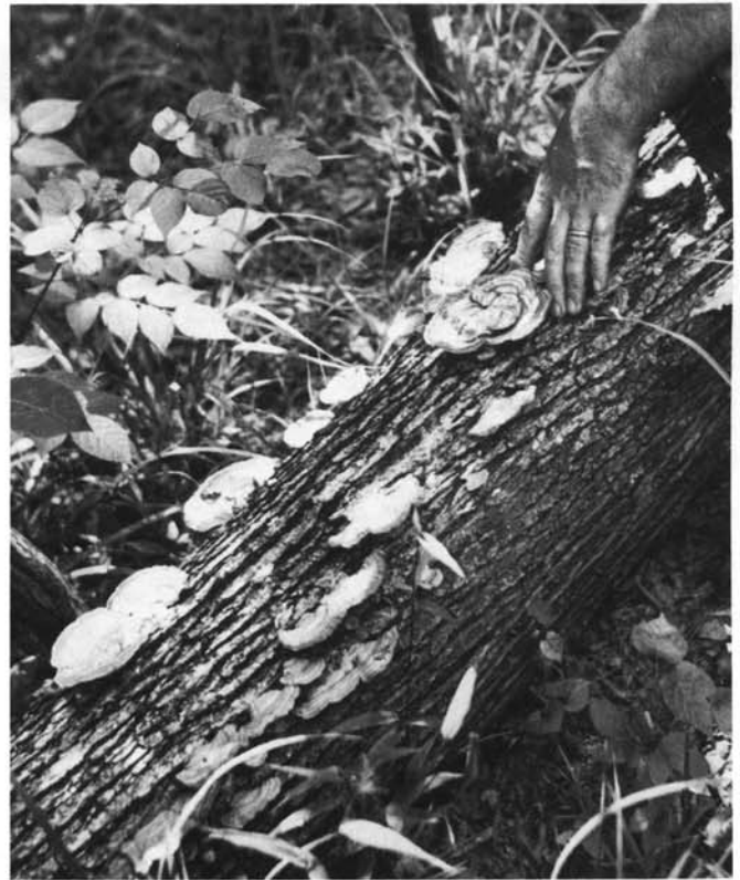
Figure 87 —Conks resulting from severe rot in red maple log. The brackets are a sign that rot has made at least the sapwood useless. The heartwood may remain sound for a considerable time, but careful examination is needed to determine the extent of rot.
