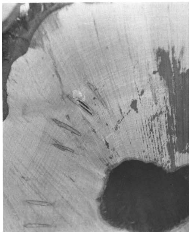
Figure 79—Flagworm or spotworm holes on red maple log.
