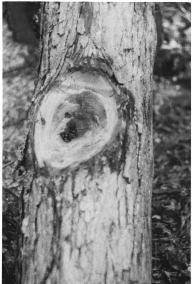
Figure 48—Knot on white oak log. A—Partly overgrown dead knot protruding through heavy callus. B—The knot cut flush shows stained, dead knot center without decay.
