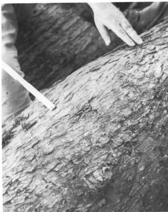
Figure 68—Surface rise on elm log.
