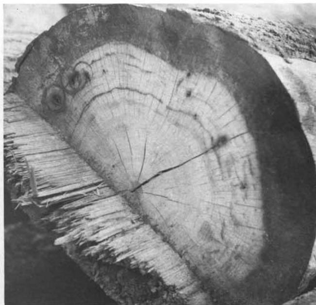
Figure 74 —Mineral streak and stain in white oak.
