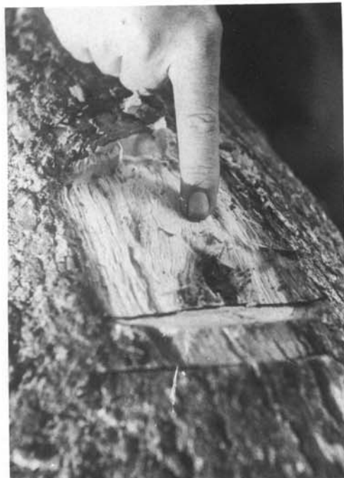
Figure 49 —Overgrown features are of fundamental importance in judging the quality of hardwood timber. A and B —Overgrowth on water oak caused by a small knot that was only recently buried. C and D —Overgrowth on blackgum caused by a deeply buried knot. E and F —Small epicormic limb on white elm leading to lumber knots. G and H —Overgrown epicormic buds surrounding an epicormic branch. I and J —Birdpeck on white oak. K and L —Large overgrowth on overcup oak caused by a wood borer.
