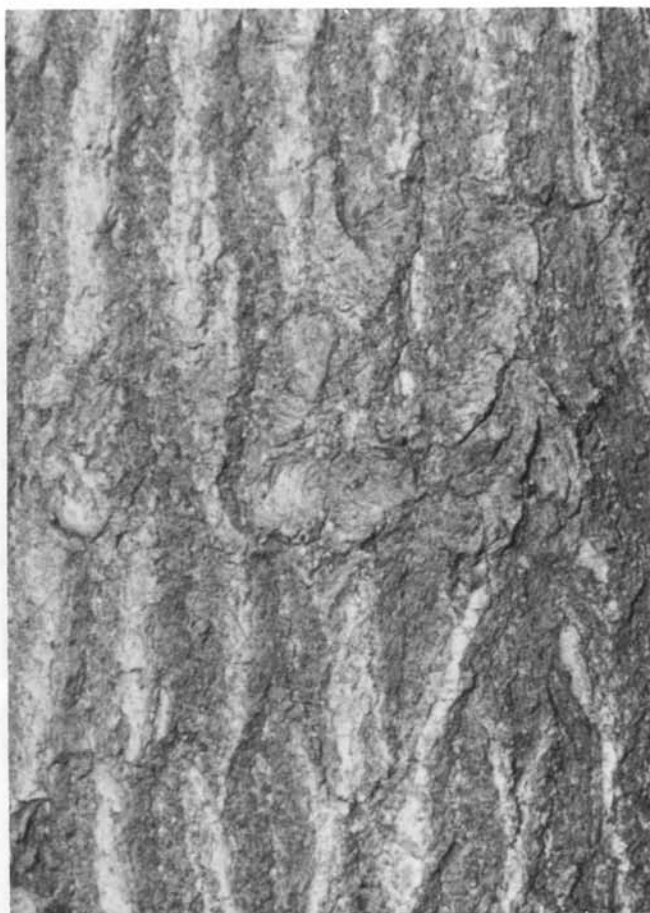
Figure 63 —Bark distortion covering a deeply buried, medium-sized knot on second-growth red oak.
