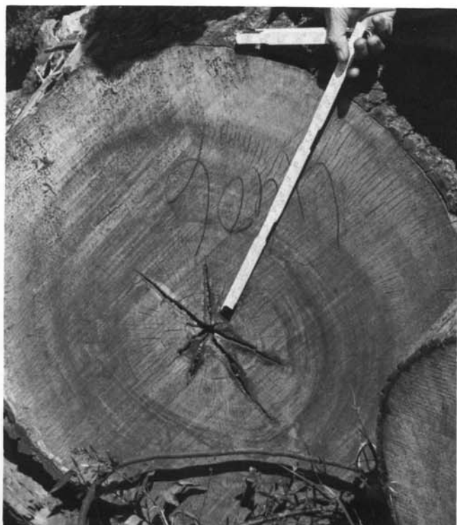
Figure 83—Spider heart on water oak log.
