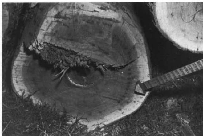
Figure 42 —End of hickory log shows stain caused by birdpeck.
