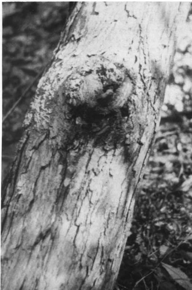
Figure 48—Knot on white oak log. A—Partly overgrown dead knot protruding through heavy callus. B—The knot cut flush shows stained, dead knot center without decay.
