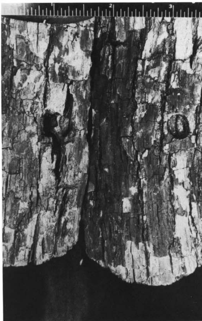
Figure 51—Overgrowths caused by borers. A—Roundheaded borer ( Goes spp.) exit holes. B—Carpenterworm ( Prionoxystus robiniae (Peck)) entrance and exit holes.
