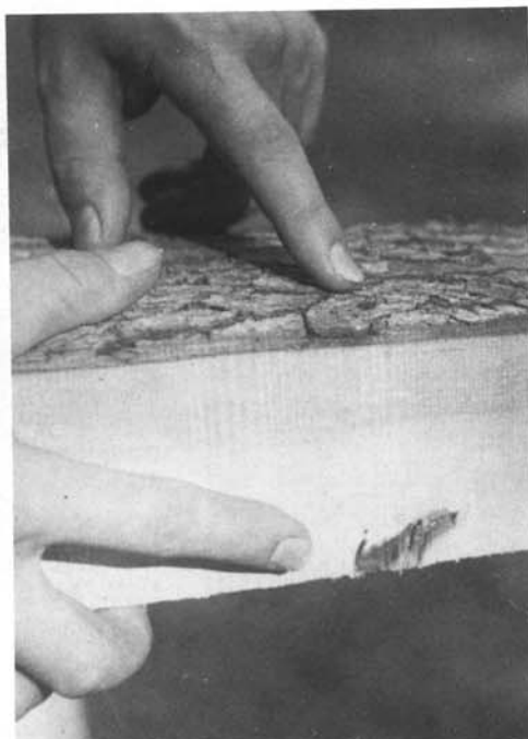
Figure 49 —Overgrown features are of fundamental importance in judging the quality of hardwood timber. A and B —Overgrowth on water oak caused by a small knot that was only recently buried. C and D —Overgrowth on blackgum caused by a deeply buried knot. E and F —Small epicormic limb on white elm leading to lumber knots. G and H —Overgrown epicormic buds surrounding an epicormic branch. I and J —Birdpeck on white oak. K and L —Large overgrowth on overcup oak caused by a wood borer.
