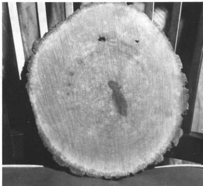
Figure 75 —Organic stain in basswood from birdpeck and a wood-boring insect.
