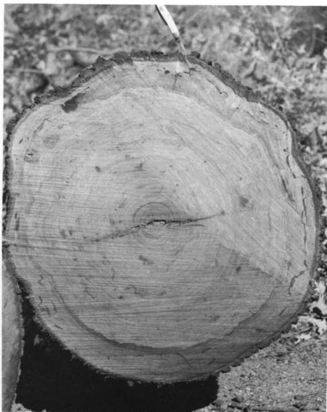
Figure 72—Grease spot in overcup oak.
