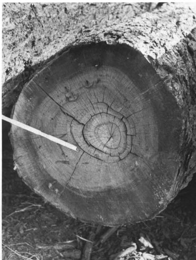
Figure 73 —Loose heart in bitter pecan ( water hickory ).
