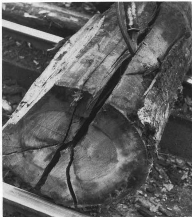
Figure 67—Split in elm log caused by careless bucking.
