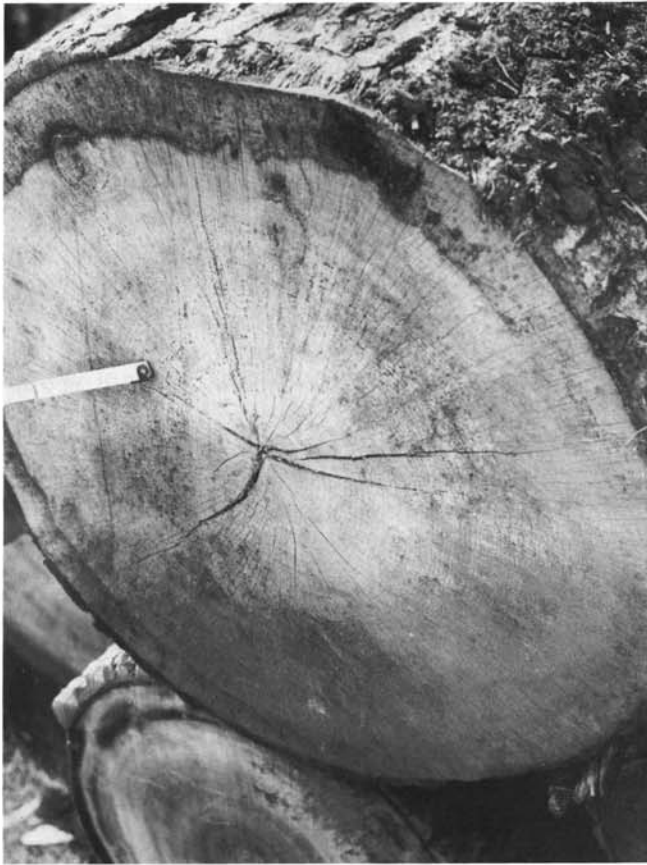
Figure 85 —Rot or decay in early stage.
