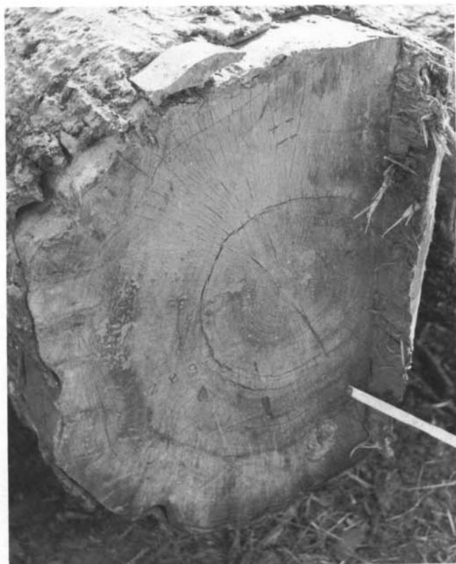
Figure 80—Ring shake on elm log.
