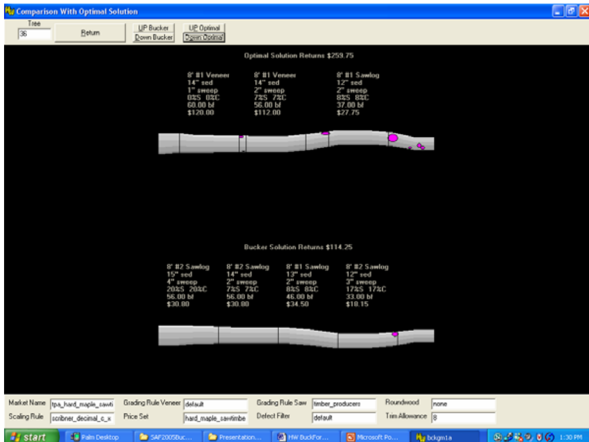
Figure 2: The HW Buck comparison page, which shows the trainee's results for comparison with the optimal bucking pattern.
